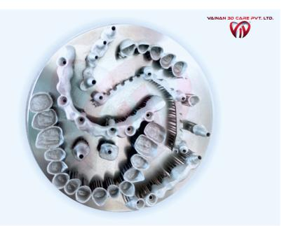
Build Plate (truprint 1000)  $\emptyset$  98 mm H - 98mm Laser Beam Spot Size  $\emptyset$  55 Microns
